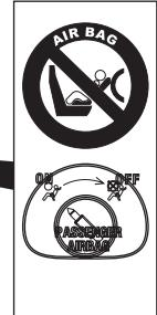
DO NOT place rear- facing child seat on the front passenger seat with airbag
